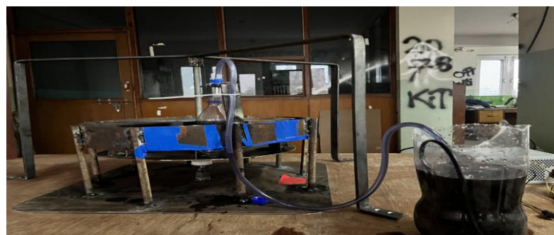
Fig. 12: Station disc with six slots and stepper motor.
