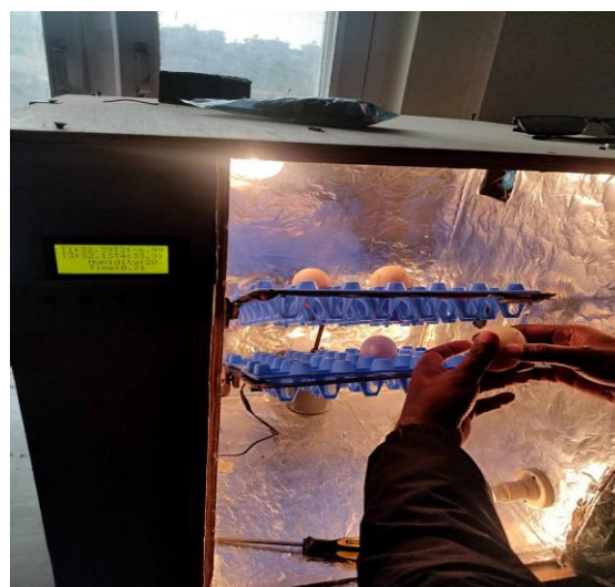
Fig. 6: Incubator and Egg placement before incubation period starts.
