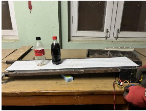
Fig. 13: Conveyor belt and reject chute assembly.
